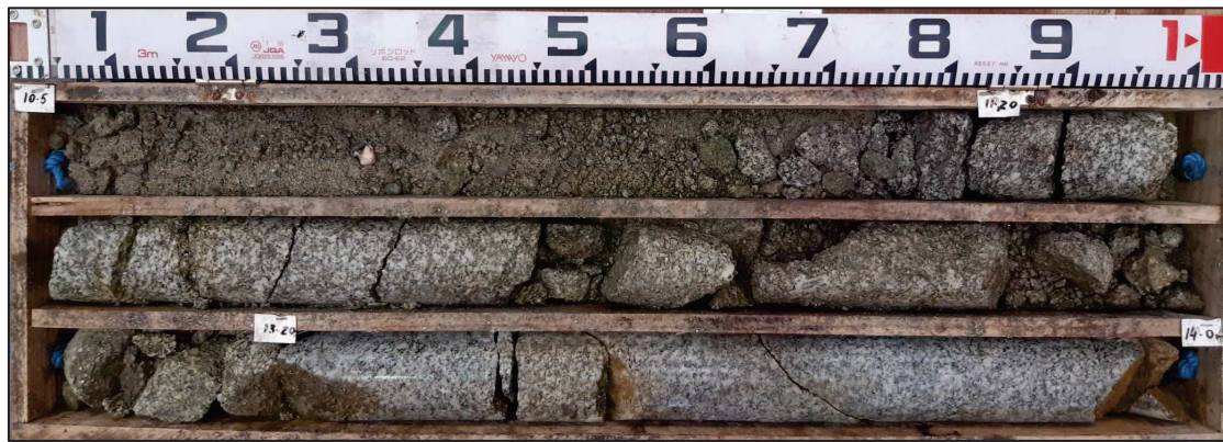
Photo 1 – Core recovery at RC02 (10.5 – 14.0 m BGL)
