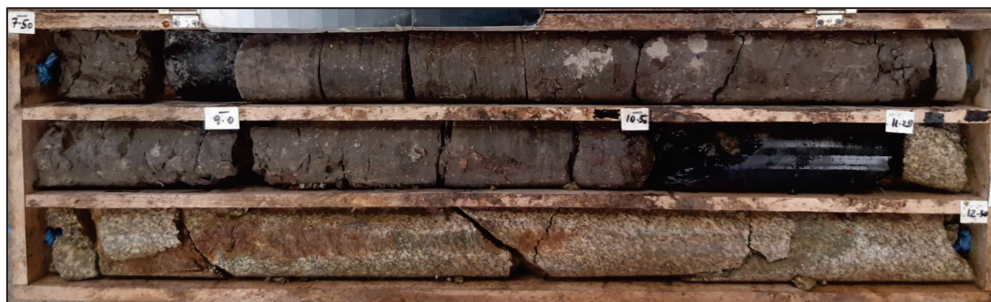
Photo 2 – Core recovery at RC07 (7.5 – 12.5 m BGL)
